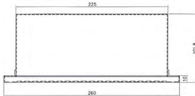
[Fig. 3-2] Top View of FTU Panel
